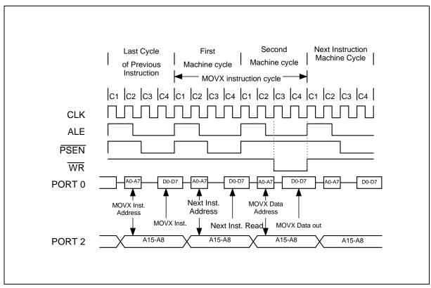
Figure 8. Data Memory Write with Stretch Value = 0
