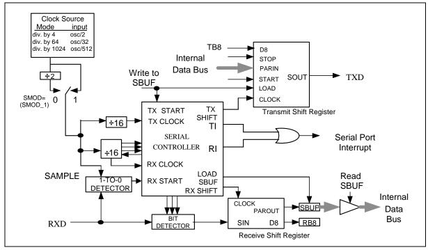
Figure 22. Serial Port Mode 2
