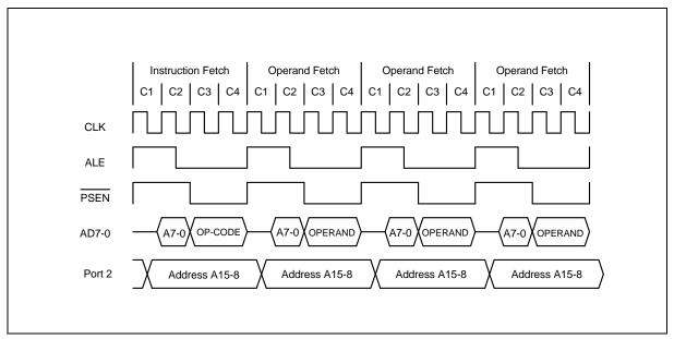
Figure 6. Four Cycle Instruction Timing
