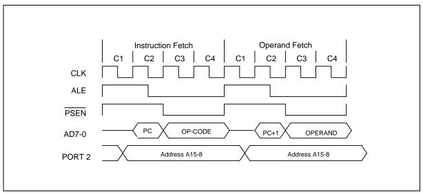
Figure 4. Two Cycle Instruction Timing
