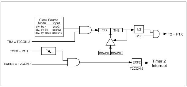
Figure 18. Programmable Clock-Out Mode
