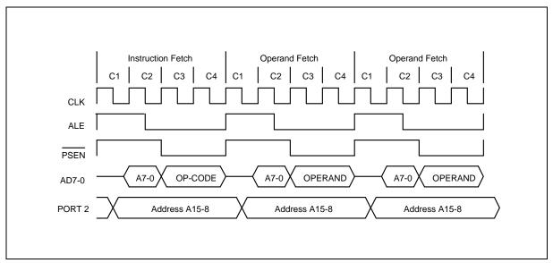
Figure 5. Three Cycle Instruction Timing
