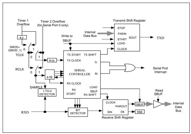
Figure 21. Serial Port Mode 1
