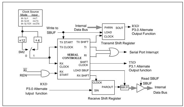
Figure 20. Serial Port Mode 0
