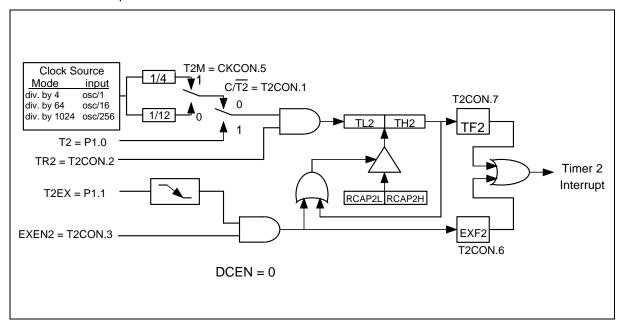
Figure 15. 16-Bit Auto-reload Mode, Counting Up
