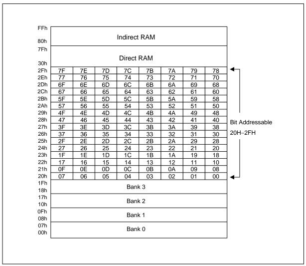
Figure 2. Scratchpad RAM/Register Addressing
