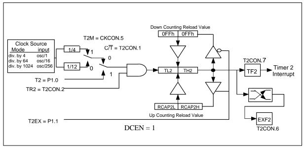
Figure 16. 16-Bit Auto-reload Up/Down Counter
