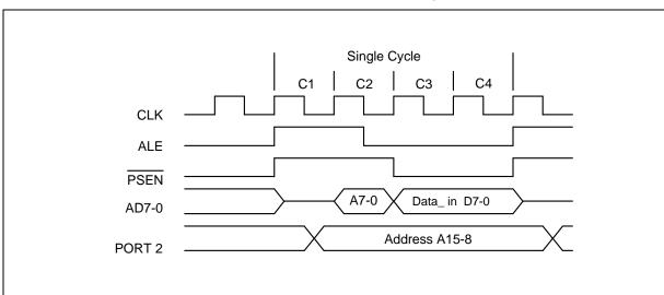
Figure 3. Single Cycle Instruction Timing
