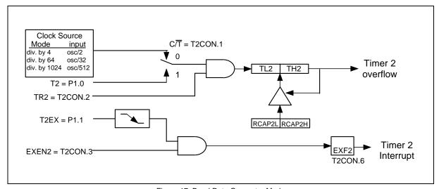
Figure 17. Baud Rate Generator Mode
