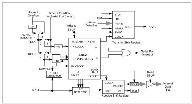
Figure 23. Serial Port Mode 3
